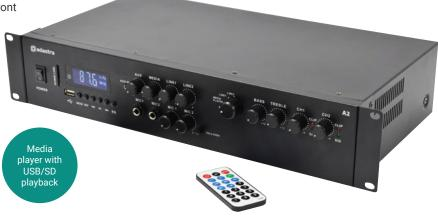
Audio source . USB/SD mp3 playback, FM tuner, BT receiver Input controls Aux, Media, Line1, Line2, Mic1, Mic2, Talkover Line output. Speaker outputs . . . . . . 4mm binding posts (2 channels) Antenna connection . . . . . . . . . . . . . . . . F type (FM tuner) Output controls . . . . . Source select, Bass, Treble, Ch1, Ch2 Dynamic range ......92dB Protection. Thermal, over-current, over-voltage, short-circuit
